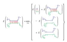
**Fig. 1.** Heuristic for reducing time complexity of IntaRNA (figure taken from (Busch et al., 2008)). The top energies are of the hybridization and the two bottom energies are for the accessibilities. The accessibilities are not additive so the contribution needs to be subtracted and then added back with the extended region.
